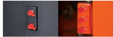
**Greasing Lubrication Ports**
